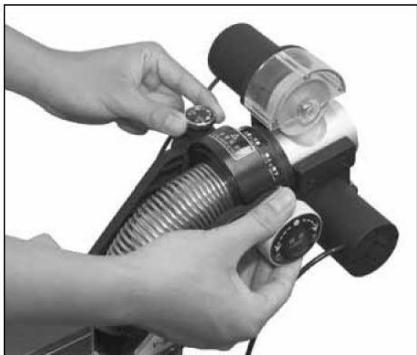
**When modulating the loop of the serve, loosen the loop lock knob with your left hand, while adjusting the loop modulation wheel with your right hand. When achieving your desired loop, lock the knob.**
