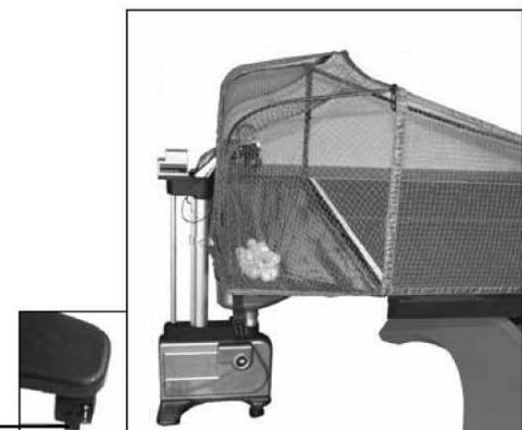
**4. Put the table tennis robot close to the edge of table. Open the wheel lock when moving the robot.**
