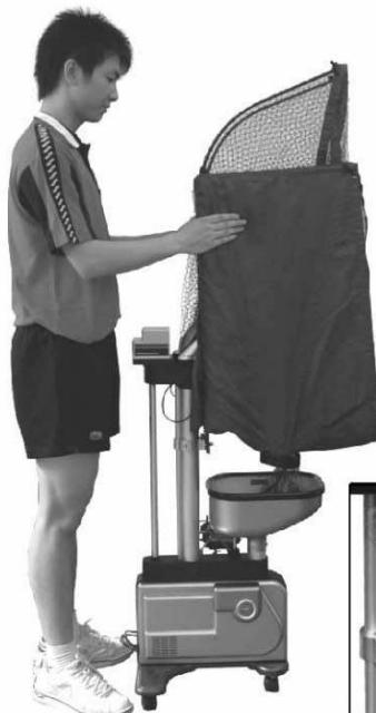
**2. Partially unfold the ball collecting net, adapt the square outlet of the net with the robot head. Insert the pin in the ball collecting net into the support frame of the robot.**
