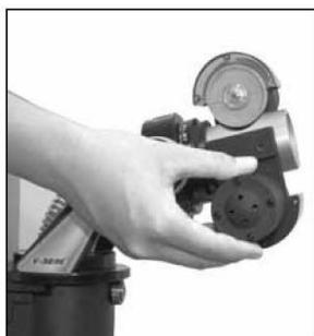
For RoboPro Genius model the spin can be selected by adjusting both the speed of top-wheel and bottom-wheel and by rotating the motor head of robot. There are totally 9 different spins you can choose from: top spin, under spin, no spin (produced by varying the speed of top and bottom wheel), left side spin, right side spin, left-side top spin, left-side under spin, right-side top spin and right-side under spin.
