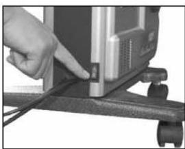
**The power switch locates at the back side of the machine body, turn the switch “on” before the use of robot and turn the switch “off” after use.**
