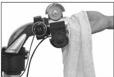
**Under normal conditions, the top and bottom wheel (friction wheel) can work for 5000 hours or longer. However, the friction wheel should be replaced after over time use. When replacing, first of all, loosen the protective cover and take out the screw at the friction wheel with a screwdriver, which is to be tightened clockwise and to be loosened counter-clockwise.**
